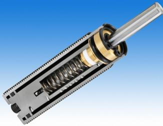
During operation the piston rod moves inside and the piston pushes the hydraulic fluid through the orifice holes, producing a resistant force. The more the piston rod enters, the more orifice holes are closed. This will reduce speed, pressure and braking remain nearly constant. This prevents the occurrence of peak power which can cause damage to products and machines.
