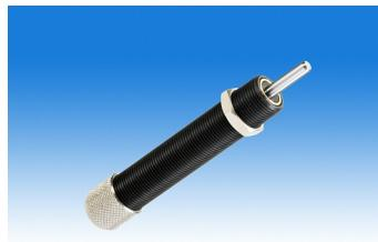
This shock absorber is designed for automatic machines, handling systems with high frequency applications. Superfine surface treatment, special seals and special oil provide a guaranteed lifetime of at least 10,000,000 strokes! The progressive characteristic ensures a smooth deceleration, even at very high driving forces.
