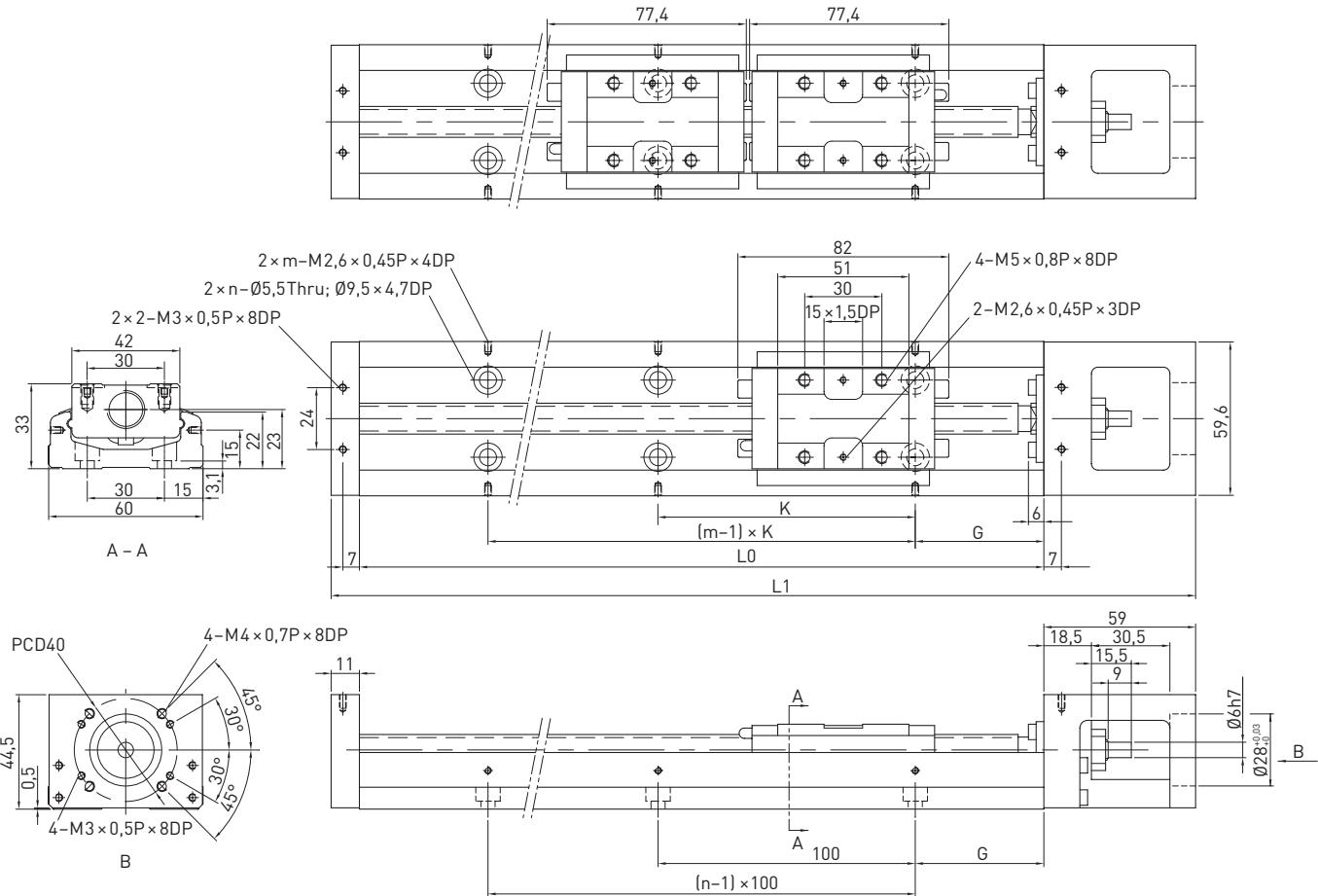
Table 2.5 Dimensions and weights of KK60 linear axes without cover, standard block
