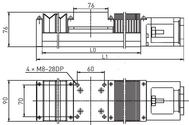
Table 2.12 Dimensions and weights of KK86 linear axes with bellow cover
