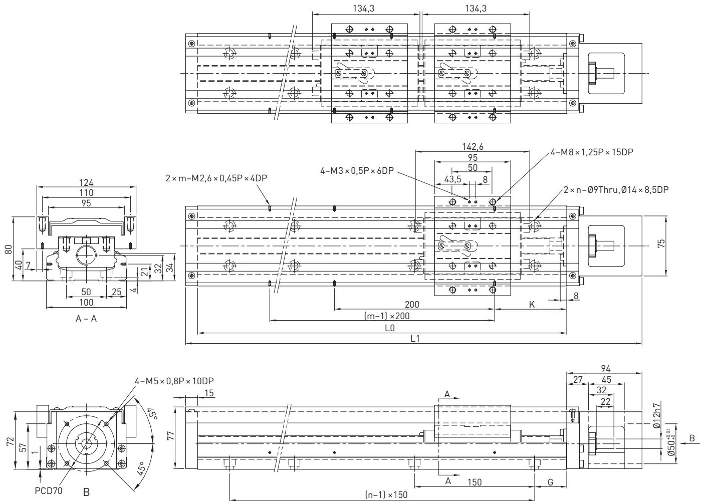
Table 2.14 Dimensions and weights of KK100 linear axes with aluminium cover
