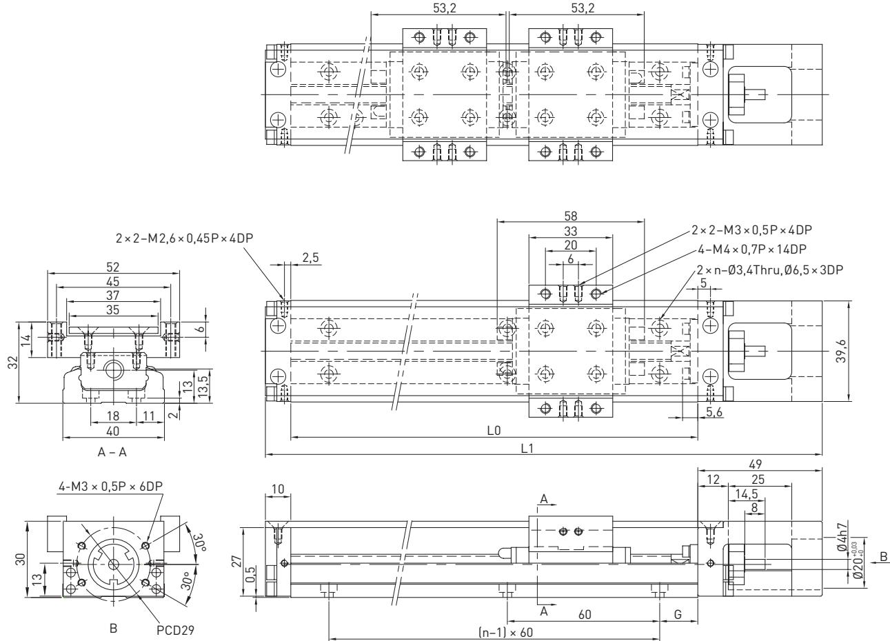
Table 2.2 Dimensions and weights of KK40 linear axes with aluminium cover
