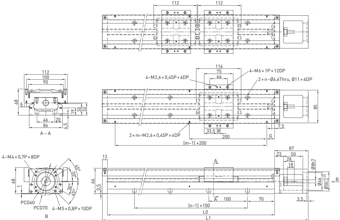
Table 2.11 Dimensions and weights of KK86 linear axes with aluminium cover
