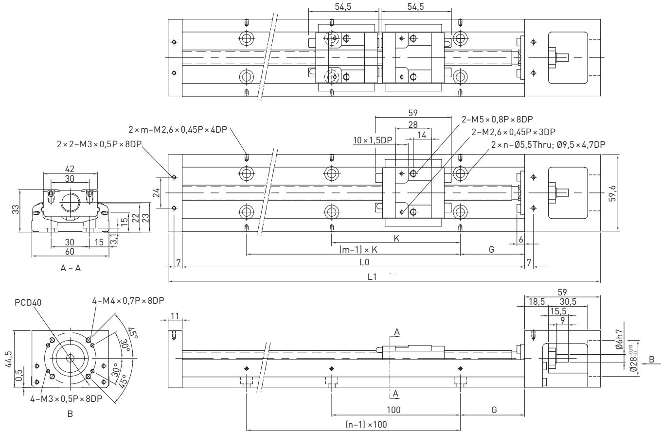
Table 2.6 Dimensions and weight of KK60 linear axes, short block
