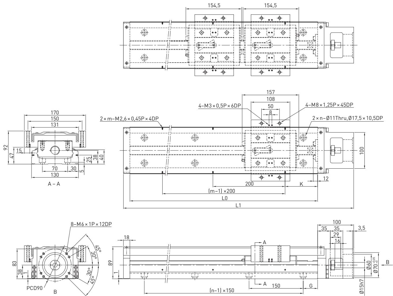
Table 2.16 Dimensions and weights of KK130 linear axes with aluminium cover
