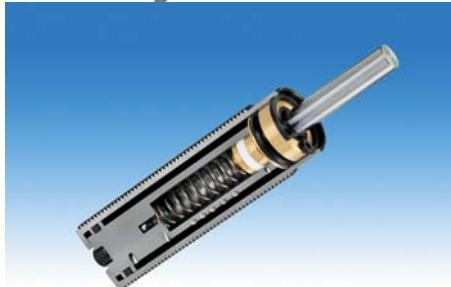
During operation the piston rod moves inside and the piston pushes the hydraulic fluid through the orifice holes, producing a resistant force. The more the piston rod enters, the more orifice holes are closed. This will reduce speed, pressure and braking remain nearly constant. This prevents the occurrence of peak power which can cause damage to products and machines.
