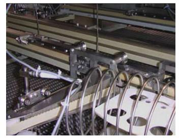
**DualVee® Washdown Wheels** protect against ingress of liquid making them ideally suited for food and beverage applications, as well as any high speed water jet cutting machinery. These applications typically require frequent bearing replacement due to the ingress of highly corrosive fluids and loss of lubrication.
