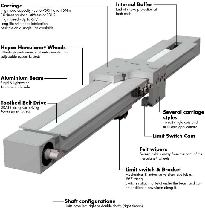
All standard PDU2 motor connection kits will fit.
