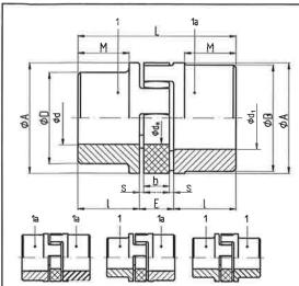
Finish-borings are made according, to the ISO system of tolerances H7. Feather key grooves are made according to DIN 6885/1. The max. angle shift is 1°30 , the Iwisting angle 3,2° at Mt nom. The operable temperature range lies between -40°C and +100°C.
