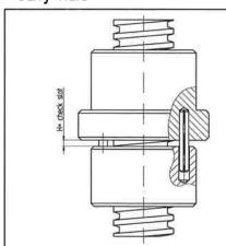
Connected with the loaded traveling nut via driving pins, the locking nut runs at idle. As the threads in the traveling nut wear it approaches the idling, unloaded and therefore unworn safety nut. The wear is ascertained by checking the slot H. When the table entry H has declined by half the traveling nut must be replaced
