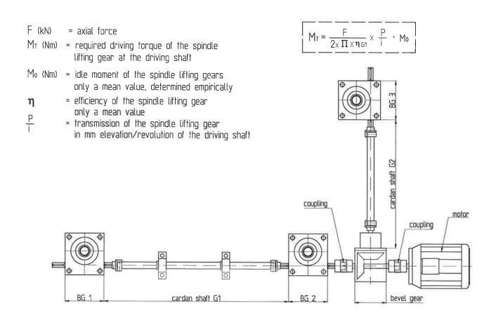
$$M_{\text{driving motor}} = M_{T BG1} \times \frac{1}{\eta_{G1}} + M_{T BG2} + M_{T BG3} \times \frac{1}{\eta_{G2}} \times \frac{1}{\eta_{K}}$$
