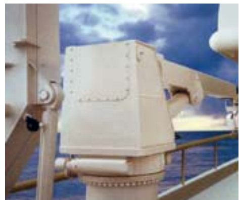
Special designed worm gear set for swing cranes on ships
